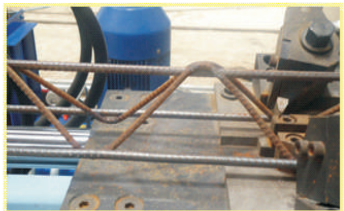
Lattice Girder Manufacturing Facility For Precast Slabs (7500 Rmt /day)
