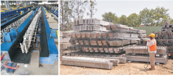
PRECAST BEAM CASTING (1800 Rmt/Day)
