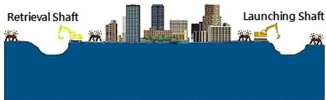
1. Excavate launching shaft and retrieval shaft
