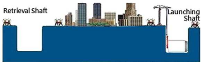
2. Assemble the TBM at the launching shaft
