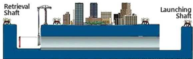
4. TBM arrives in the retrieval shaft to be dismantled for transportation
